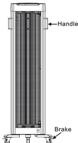
1. Before moving the device, make sure the power cable is disconnected from power socket and the wheel brake is released. To release the brake, push the brake lever up with your foot.
